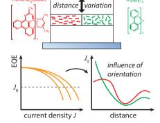
The efficiency roll-off of organic lightemitting diodes is studied by varying the distance between emitter and metal cathode. Roll-off is found to depend on the orientation of the emitter molecules, which can be explained by measurements and modeling of the triplet decay rate. Simulations of the roll-off behavior give further insight into the principles of efficient stack design.
