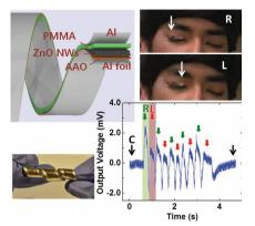
Ultrathin piezoelectric nanogenerator is developed as active or self-powered sensor for monitoring local deformation on a human skin. The nanogenerator which detects the motion of the eye ball underneath can be effective in monitoring sleep pattern, tiredness, brain activity, and spirit status of a person, as well as any biological associated skin deformation.
