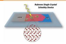
The photovoltaic effect at the Schottky interface of a rubrene single crystal and Al or LiF/Al electrodes in lateral ITO-rubrene-Al and ITO-rubrene-LiF/Al device configurations is demonstrated and explained based on constructed energy band diagrams of the heterostructures.
