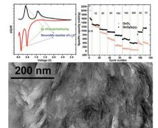
A GeO<sub>x</sub>/reduced graphene oxide (RGO) composite, where amorphous GeO, (1.01 < x < 1.07) nanoparticles are in intimate contact with well-dispersed RGO sheets, is successfully synthesized via a facile one-step reduction approach. The introduction of conductive RGO sheets into germanium oxide is a simple but effective strategy for enhancing the reversible utilization of Li<sub>2</sub>O and improving rate capability for Li+ storage in germanium oxides.
