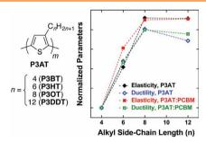
This paper describes the large effect of small changes in a structural characteristic—the length of the alkyl side chain—on the elasticity and ductility of conjugated polymers. Measurements of tensile modulus are complemented with measurements of ductility. These experiments could influence the selection and design of new organic semiconductors in flexible and stretchable applications.
