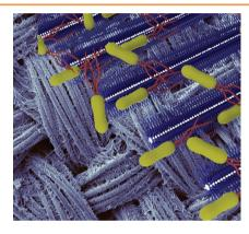
The synthesis of Ag-tetracyanoquinodimethane (TCNQ) nanowires of extremely high aspect ratios (>3000) supported on a metallic silver fabric is reported. These Ag/AgTCNQ fabrics show higher antimicrobial performance against both Gram negative and Gram positive bacteria than pristine Ag fabrics. This study extends the applicability of metal-TCNQ charge transfer complexes beyond electronics applications and opens up new avenues towards flexible electronics.
